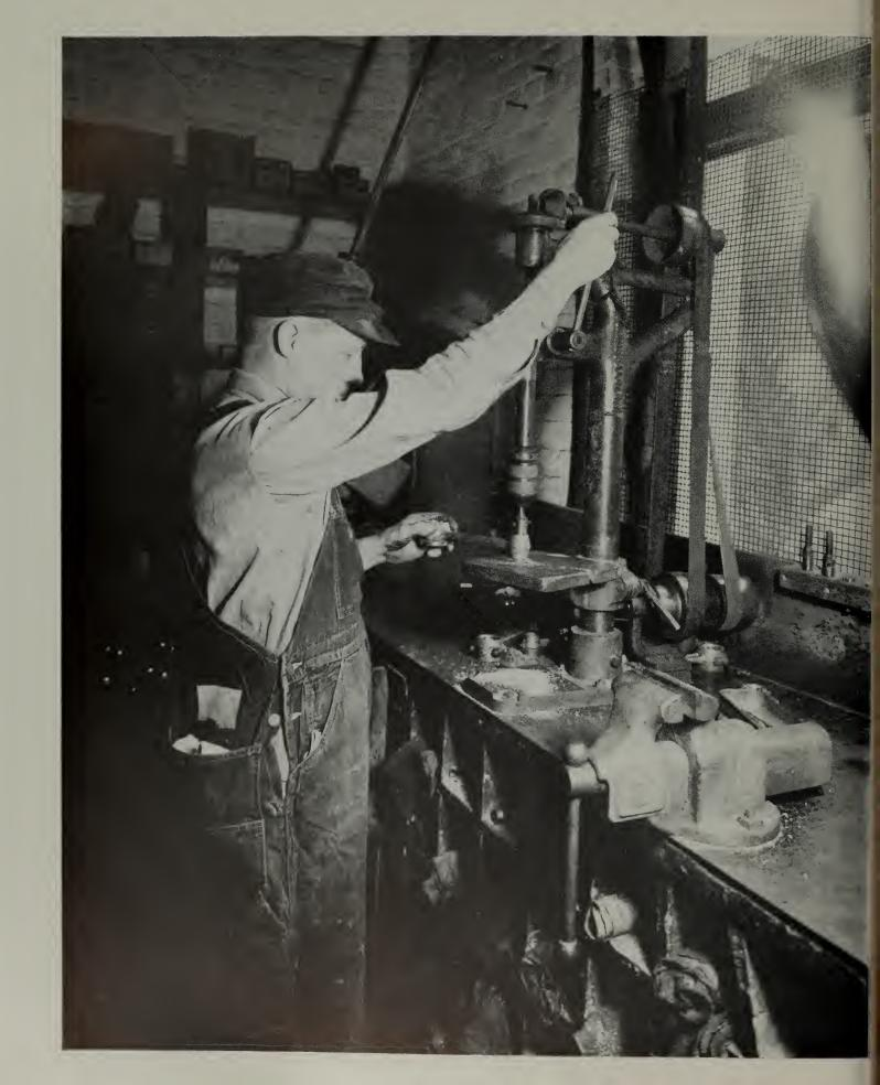
Model A Ford connecting rods are fitted with a very thin bushing which becomes somewhat damaged and burred when being pressed in by the arbor press shown in Picture 26. This is corrected by placing the connecting rods in a bench drill press in which a chamfering tool is used as shown in the above picture.
